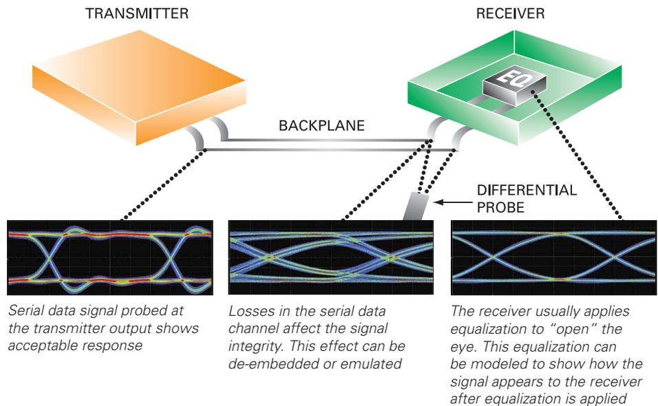
Serial data signal probed at the transmitter output shows acceptable response
