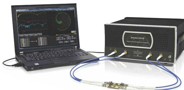
*The SPARQ can perform all serial data compliance tests currently made with TDR or VNA instruments – only easier.*
