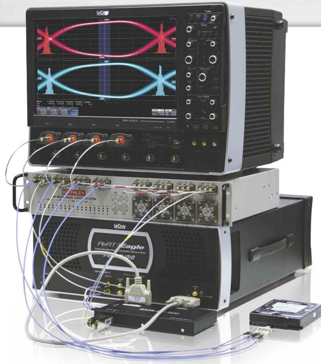
The combination of the SDA 8 Zi-A Serial Data Analyzer, the PeRT<sup>3</sup> and the SPARQ provides the most comprehensive solution for serial data compliance testing. These three pieces of equipment enable a full suite of physical layer compliance testing and debugging ability that will guarantee the best signal integrity for your serial data signals.
