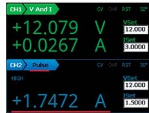
Pulse Current Measurement for PPH-1503D
