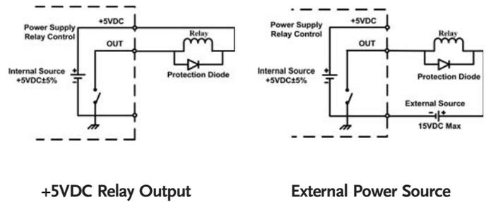
Using the +5VDC relay output to drive an external relay. Ensure the current does not exceed 150mA.
