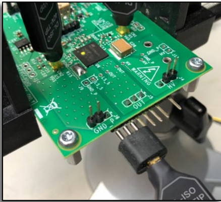
DL-ISO with flexible interfaces to DUTs
