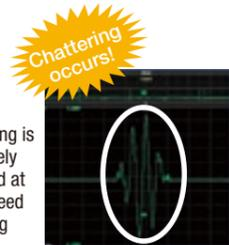
Chattering is accurately captured at high-speed sampling. Check the frequency of occurrence at low -speed sampling
