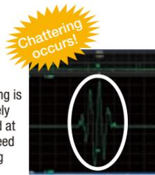
Chattering is accurately captured at high-speed sampling. Check the frequency of occurrence at low -speed sampling
