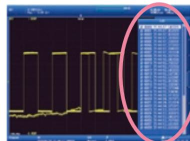
You can display all past waveforms, and view a list of acquisition times.
