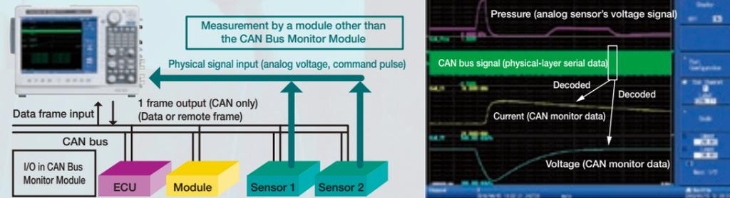
Data to be acquired using a bus monitor module (720240 or 720241) can be specified not only in digital code (hexadecimal or numeric), but also loaded from a network definition file (CAN DBC or LIN LDF).
