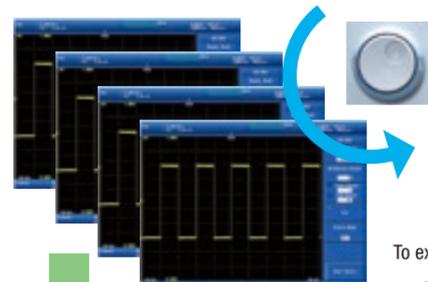
Use the jog shuttle to display past waveforms
