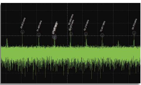
X-Stream II fast throughput streaming architecture makes difficult analysis and deep insight possible. Above, an FFT is applied to a 50 Mpts waveform to determine root cause failure. The high frequency resolution this provides enables deep insight into signal pathologies.
