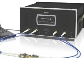
The SPARQ signal integrity network analyzers connect directly to the device under test (DUT) and to PC-based software through a single USB connection for quick, multi-port S-parameter measurements.
