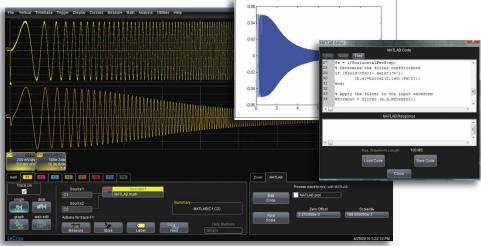
XDEV Customization software package being used to implement a 1 MHz Butterworth filter using MATLAB<sup>®</sup>.
