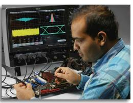
Capture 5 ms (100 Mpts) of low-speed and high-speed waveforms. Decode low and high speed serial data signals.Easily zoom, and validate timing relationships between signals.
