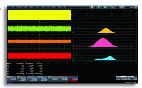
Capture a single clock channel (yellow) and display Track graphs and Histograms simultaneously of multiple jitter parameters.
