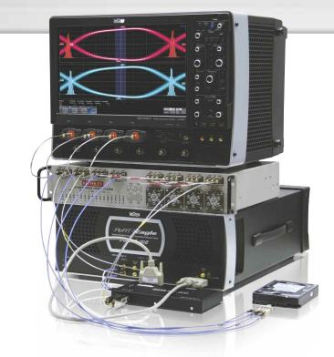
The combination of the SDA 8 Zi-A Serial Data Analyzer, the PeRT<sup>3</sup> and the SPARQ provides the most comprehensive solution for serial data compliance testing. These three pieces of equipment enable a full suite of physical layer compliance testing and debugging ability that will guarantee the best signal integrity for your serial data signals.
