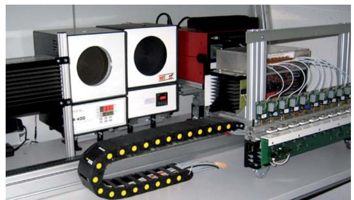
Automated calibration stations at Optris GmbH
