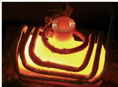
optris CTlaser 1M/2M devices for the use at induction hardening.
