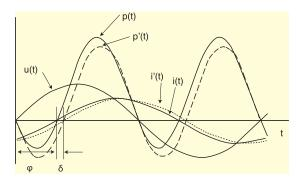
$U_{(1)} = U_{pk} sin(\omega t) \quad i_{(t)} = I_{pk} sin(\omega t - \phi) \quad i'_{(t)} = I_{pk} sin(\omega t - (\phi + \delta))$
