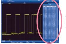
You can display all past waveforms, and view a list of acquisition times.
