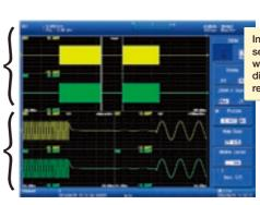
Instantly zooms 1 second (100 ms/div) even when the main screen is displaying 20 days of recording (2 days/div)
