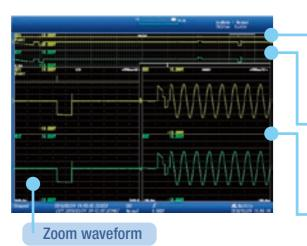
You can record up to 5,000 phenomena of high speed trigger measurements (up to 100 MS/s) at a record length of 5-500 kPoints while taking trend measurements at up to 100 kS/s.
