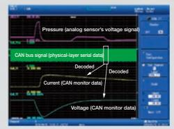
Data to be acquired using a bus monitor module (720240 or 720241) can be specified not only in digital code (hexadecimal or numeric), but also loaded from a network definition file (CAN DBC or LIN LDF).
