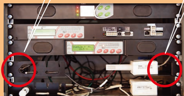
F5300 - Teflon (PTFE) sensor cover (white colour), with increased resistance against splashing water, non-absorbent surface, does not rust. Porous size 25µm. Temperature range -40°C to +125°C.
