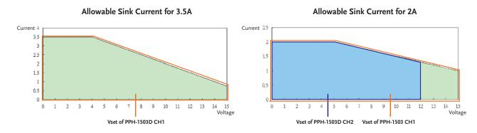
The Diagrams Show Voltage Setting Values and Allowable Sink Current for 3.5A and 2A of PPH-1503/PPH-1503D
