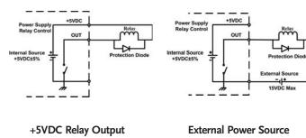
Using the +5VDC relay output to drive an external relay. Ensure the current does not exceed 150mA.
